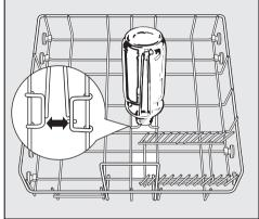
■ Place the insert into the lower basket as shown in the illustration. If placed anywhere else, water will not reach all surfaces. The item will not be properly cleaned.
